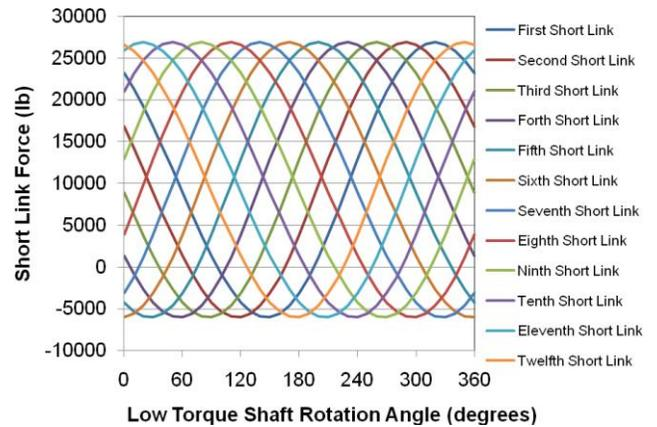
**Fig. 21-Short Link Forces for One Rotation of the Low Torque Shaft**
