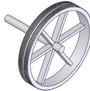
**Fig. 13-High Torque Shaft and Two Spur Gears**
