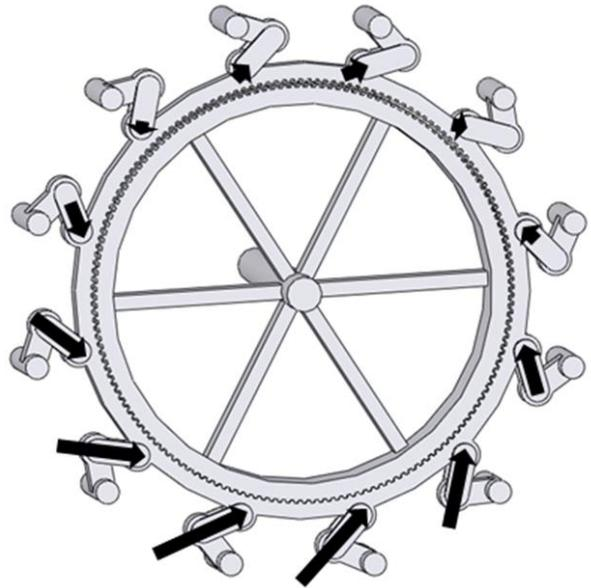
**Fig. 20-Short Link Forces for One of the Two Translating Gears**
