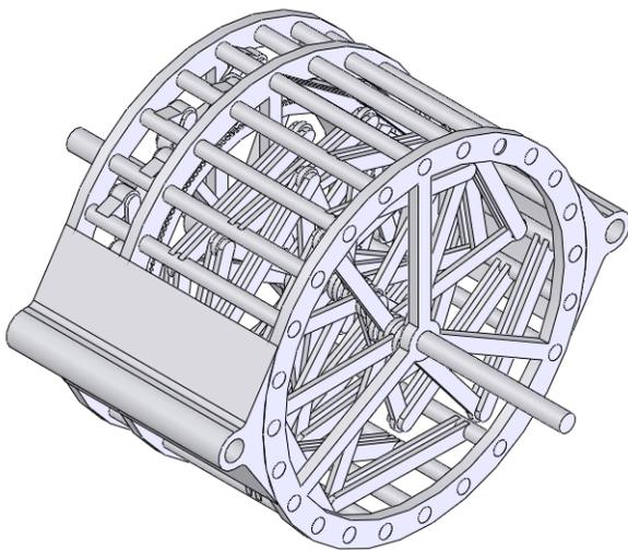
**Fig. 12-1.6 MW Eclipse Gearbox**
