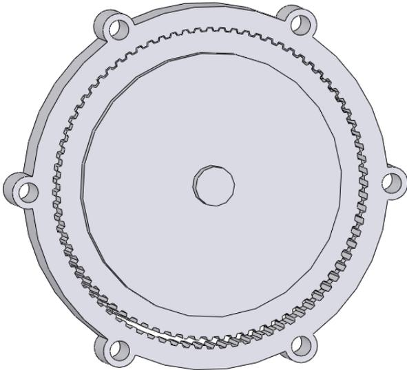
**Fig. 22-Torque Distributed Over Several Gear Teeth**
