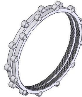
**Fig. 14-Two Translating Gears**
