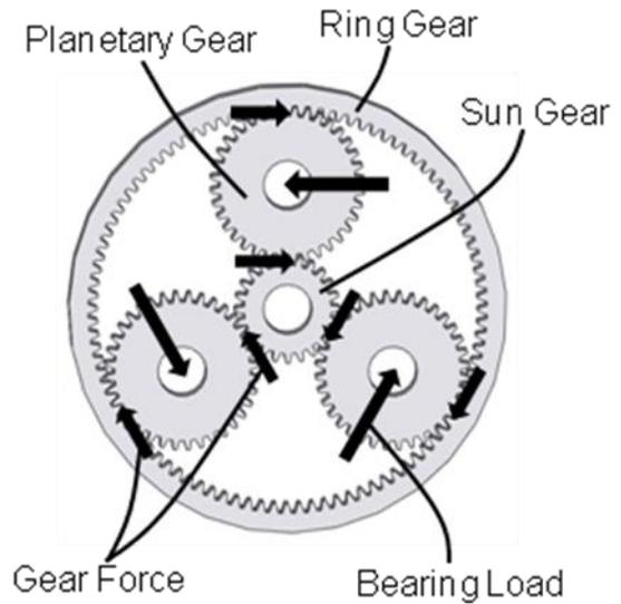
**Fig. 4-Planetary Gear Set Loads**
