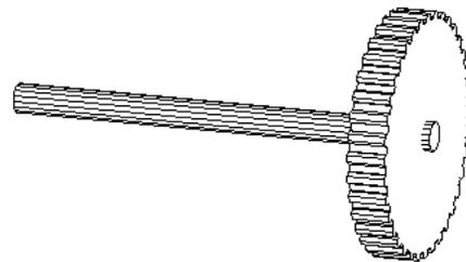
**Fig. 5-High Torque Shaft and Spur Gear**
